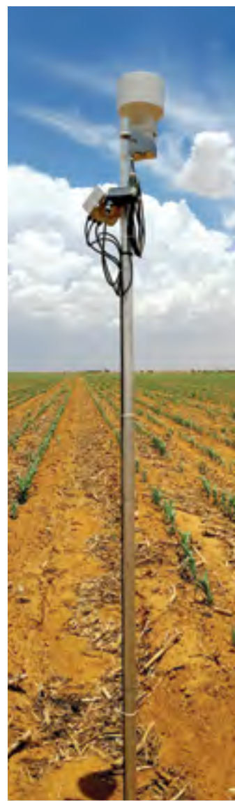
Soil moisture probe placed by Omnia
